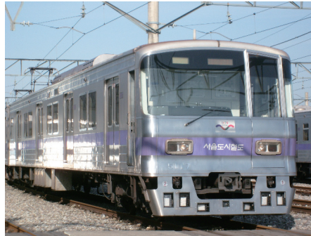
▶ Front part of a train used for the Tunnel Monitoring System; mounted on the bottom are Cameras and infrared lighting are installed on the front part of the train to monitor the dark tunnels.
